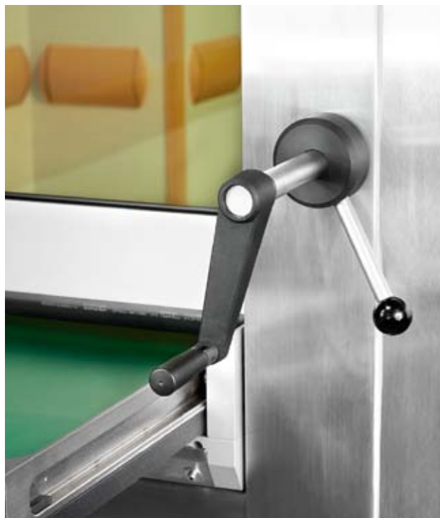
Manual emergency movement
