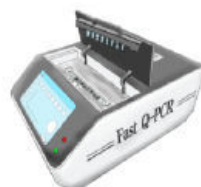
12. Put the PCR 8-tube strip into UltraFast QPCR Instrument HC800, choose the program to run
