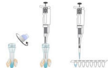
7. Unscrew the cap, pipette 20µL of the RNA sample into PCR reaction tube
